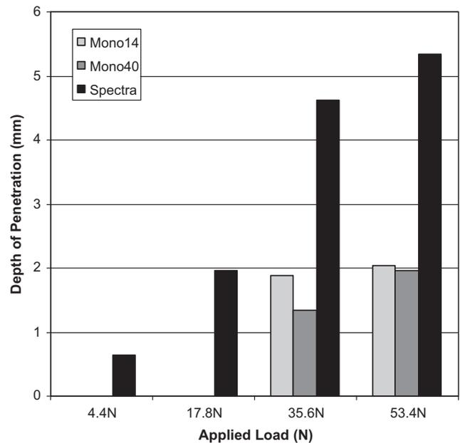
Fig. 4. Depth of epidermal penetration versus applied load for three types of fishing line. Spectra® was the most abrasive of the line types tested with penetration depths more than twice that of the monofilament lines under similar load conditions.
