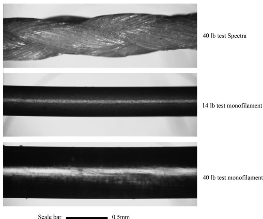
**Fig. 2.** Line types tested: 40 lb test Spectra<sup>®</sup>, a similar diameter (14 lb test) monofilament, and a similar strength (40 lb test) monofilament. Note the smooth texture of the monofilament twines compared with the convoluted surface of the braided Spectra twine with its microfilament strands. Images taken at 40× magnification.
