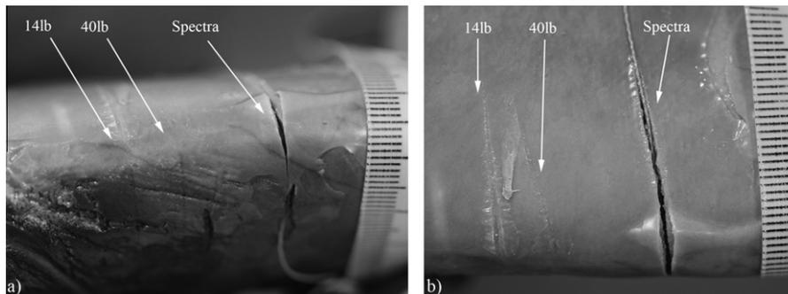
Fig. 3. Abrasion resulting from a unidirectional 3.1 m draw of line across a dolphin fluke sample under a 17.8 N load: (a) view from leading edge of fluke; (b) view of flat plane of fluke blade. Both 14 and 40 lb test monofilament lines left a superficial indentation while the Spectra® line cut through the epidermis and became embedded in the dermal layer. Scale bar on flexible ruler is 1 mm.
